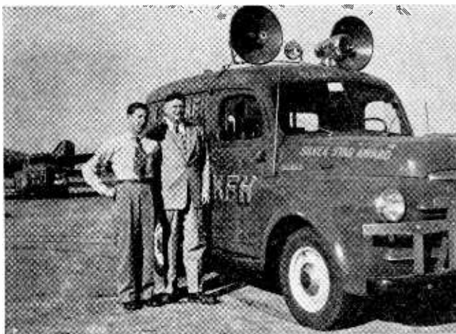
Mobile Unit KA-7765, 26.21 mcs., 26.31 mcs., and 26.41 mcs., F.M. Antenna for transmitter shown in folded position. NRI Grad T. L. Kidd, (right) chief engineer of KFH & KFH-FM, and Don Munson (left) are shown in the photograph.
